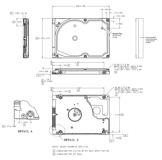
Figure 4. Mounting dimensions-top, side and end view
