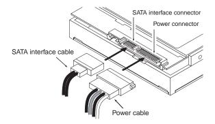
Figure 3. Attaching SATA cabling
